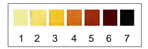
Oil should be changed before it has reached color 4. If the oil is allowed to degrade to the extent that colors 6 & 7 are reached, the pump may have suffered damage & should be fully serviced prior to re-use.
